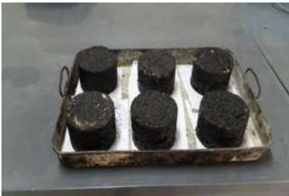
Fig. 1. Marshall Molds at different percentages of bitumen
